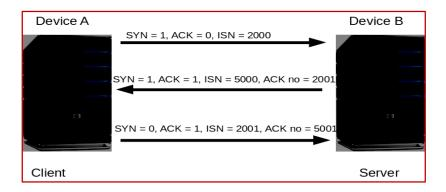
**Step 1**. Device A (Client) sends a TCP segment with SYN = 1, ACK = 0, ISN (Initial Sequence Number) = 2000. Refer TCP header
