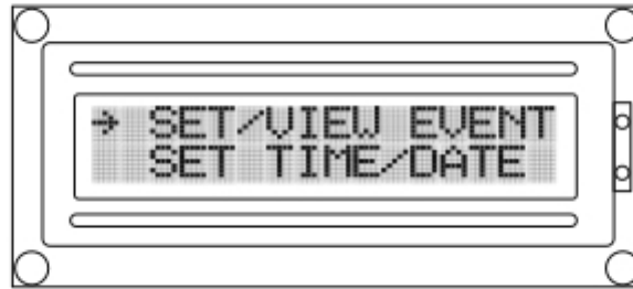
Fig 5 5: Config Screen. You get this screen by pressing either UP or Down Key. If left Idle for 5 Secs, Should go back to Default Screen. Long press of UP should provide the next screen
