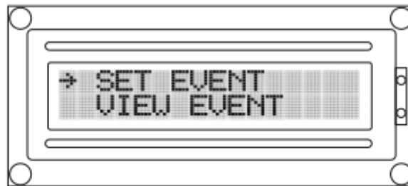
Fig 5 6: Config Set / View Event Screen. Long press of UP key should provide the next screen. Long press of DOWN key should go back to previous screen
